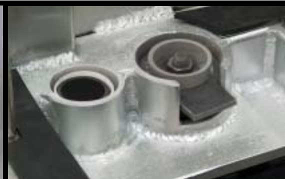
FMS mounting system extends service life of the body
