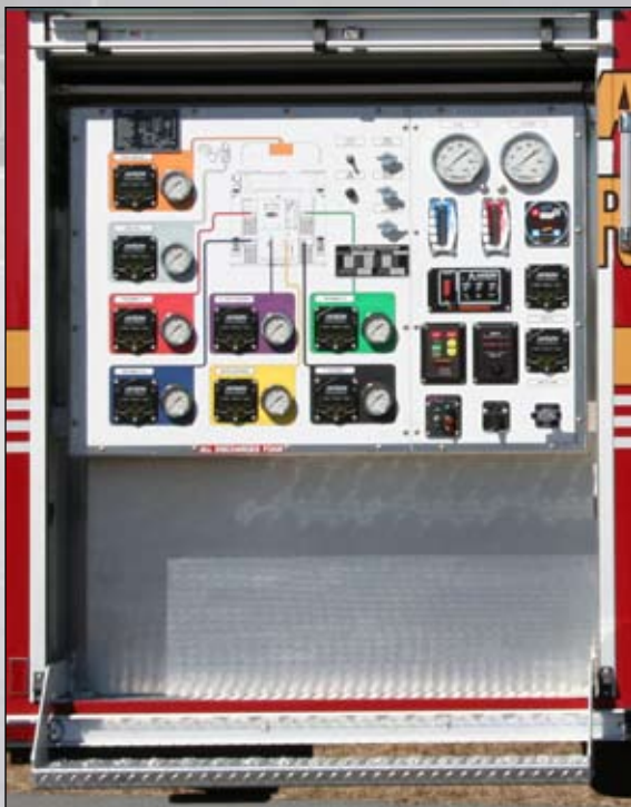
Driver or officer rear side pump operator position with manual or electric controls.
